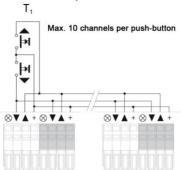
Local control with status display: Only one LED allowed. Do not link LED connections to each other.
